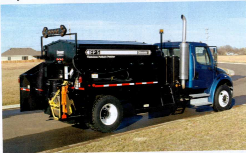
Hotboxes allow contractors to keep mix heated all day or overnight, which saves on costs and reduces waste.
